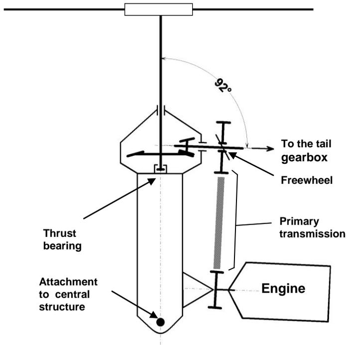
The primary transmission is composed of a pulley directly bolted to the engine output flange, a poly-V belt transmitting the power, and an upper pulley connected through a freewheeling unit to the gearbox input.
