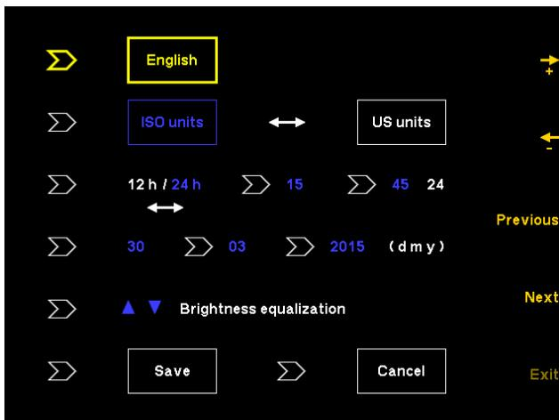
Note: Brightness equalization with NAV. light ON adjusts relative instrument panel lighting. With NAV. light OFF, it adjusts relative EAN brightness.
