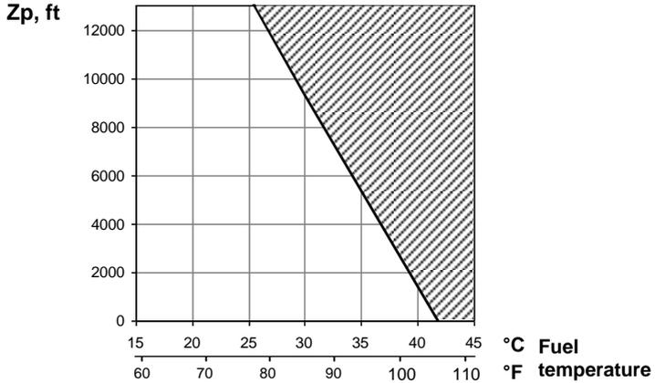
**Note:** Exceeding this flight restriction will result in engine roughness, then loss of power.
