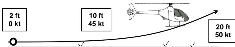
**Note 1:** Take-off is possible without increasing power in case of a very slow acceleration on hard surface.
