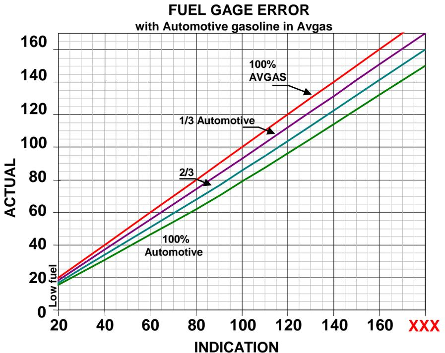
**Note:** Above 150 liters in the tank, measured value may exceed 180 liters, therefore leading to **XXX** fuel gage indication for a maximum of 30 minutes of flight. This will lead to a warning on the test page at the beginning of the following flight.
