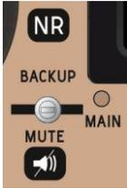
Backup mode: BARC is powered directly by the battery. Central green light is active.
