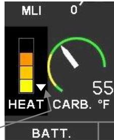
**Note 1:** During ground run or at low power setting, with a warm engine, T. induction may be biased by carburetor body heat radiation. For this reason, a brick can appear whereas the heating valve is closed.
