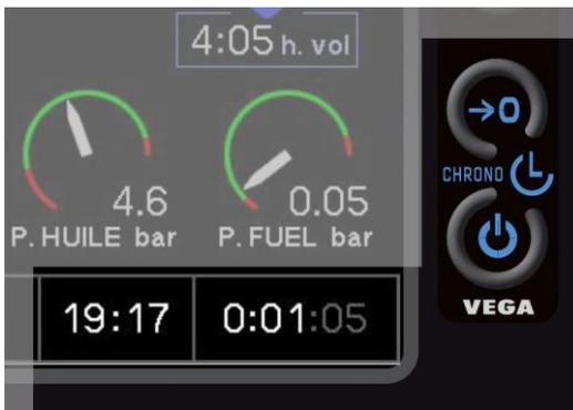
The clock is a continuous display. 12 or 24 - hour format can be selected through configuration page.
