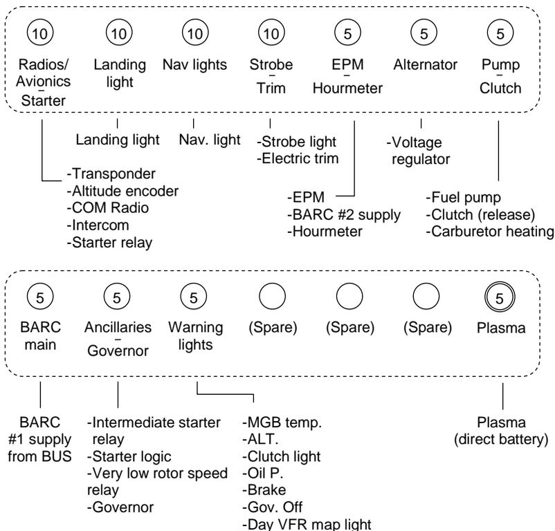
*The breakers value is given in amperes on the breakers.*
