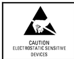
*The GTX 328 contains static sensitive components. Observe proper ESD procedures while repairing the unit. Do not replace assemblies with the unit turned on. To avoid damaging the circuit boards and assemblies, the following procedures should be carefully followed.*
