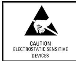
The GTX 328 Transponder contains static sensitive components. Observe proper anti-static procedures when testing the unit.
